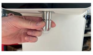
2. Put all stainless steel items into milk vessel with cleaning agents used in daily cleaning cycle.
